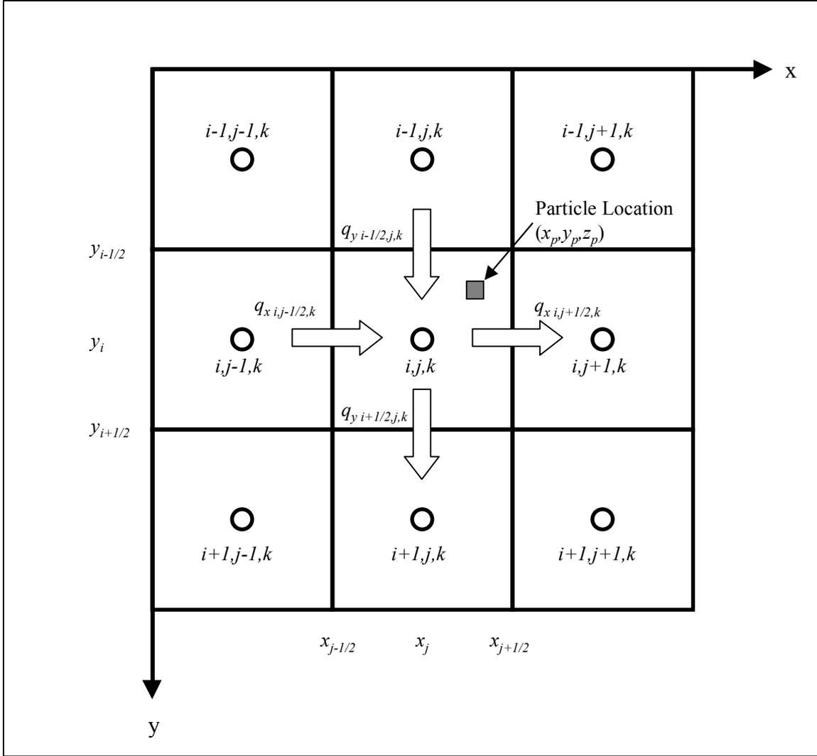
Figure 15. Velocity interpolation scheme used in particle tracking
